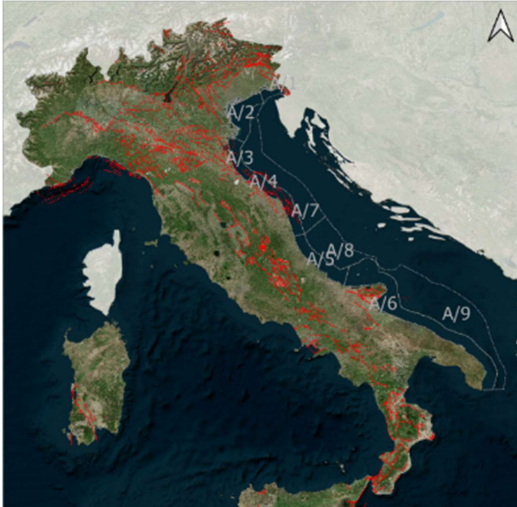
Figure 4.56 -Adriatic Maritime Sub-Areas and Catalogue of Capable Faults in Italy ITHACA (ITaly HAZard from CAPable faults. http://sgi2.isprambiente.it/ithacaweb/viewer/ ), Catalogue of active and capable faults in Italy: capable faults (activated in the last 125,000 years) and potentially capable (active in the last 2 million years), known in Italian literature (Processed by SOGESID 2022).
